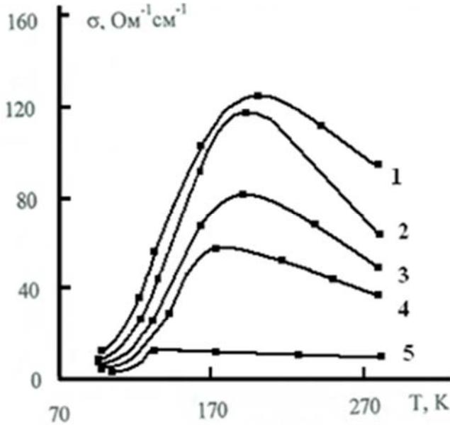
Fig. 5. Temperature dependence of electrical conductivity of Pb<sub>1-x</sub>Mn<sub>x</sub>Te thin films irradiated at  $\Phi = 2\cdot 10^{15}\text{cm}^{-2}$ : 1)  $x = 0$ , 2)  $x=0.01$ , 3)  $x=0.02$ , 4)  $x=0.04$ , 5)  $x=0.05$ .
