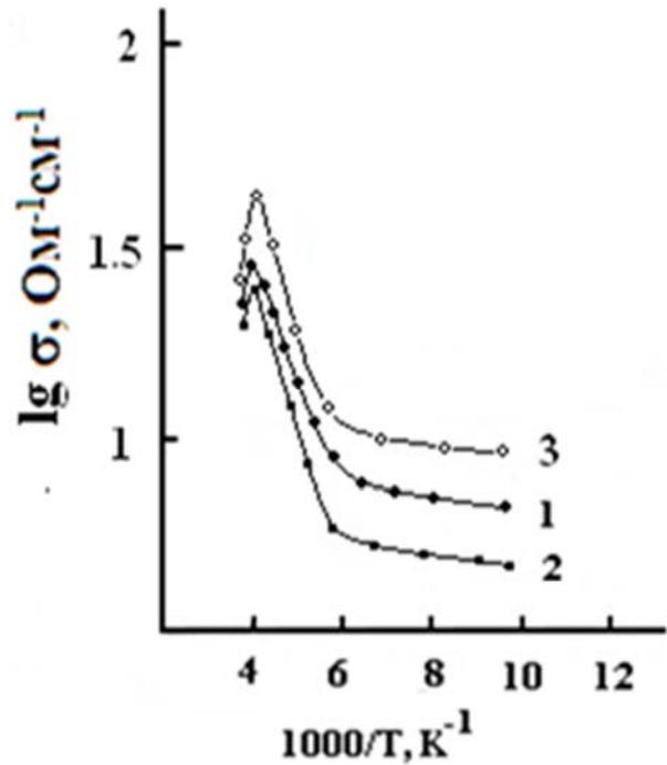
Fig. 7. Temperature dependence of electrical conductivity of Pb<sub>1-x</sub>Mn<sub>x</sub>Te ( $x=0.04$ ) thin films irradiated at 1.  $\Phi = 0$ ; 2.  $\Phi = 2\cdot 10^{15}\text{cm}^{-2}$ ; 3.  $\Phi = 10^{16}\text{cm}^{-2}$ .
