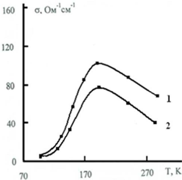
Fig. 6. Temperature dependence of electrical conductivity of Pb<sub>1-x</sub>Mn<sub>x</sub>Te ( $x=0.02$ ) thin films 1)  $\Phi = 0$ ; 2)  $\Phi = 2\cdot 10^{15}\text{cm}^{-2}$ .
