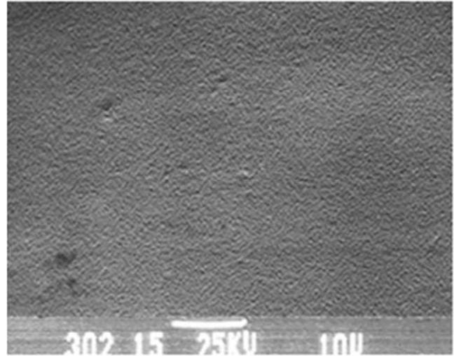
**Fig. 1.** Electron microscopic patterns the surface of  $Pb_{1-x}Mn_xTe$  ( $x=0,01$ ) thin films a) before compensation by Te at  $T_{no0} \geq 680$  K, b) after compensation by Te at  $T_{Te} = 370-460$  K.
